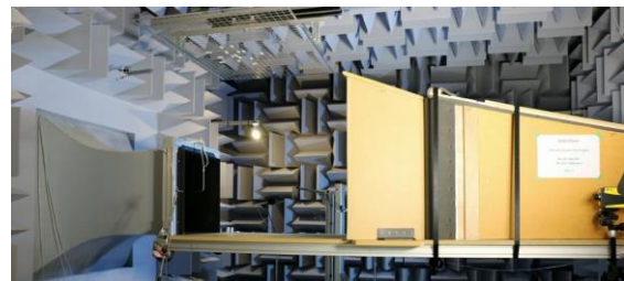
Anechoic wind-tunnel BETI: Left: general view; right: open test-section.
